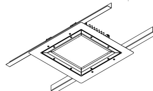
PETROL 2.0 luminaire with a cover to be mounted on crossbars and ceiling (no screws for ceiling mounting included).
