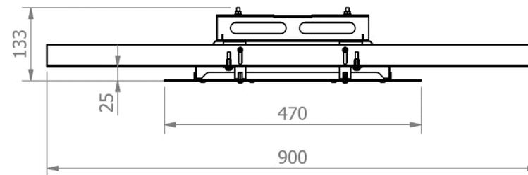
PETROL 2.0 luminaire with a cover to be used only when mounting to crossbars.
